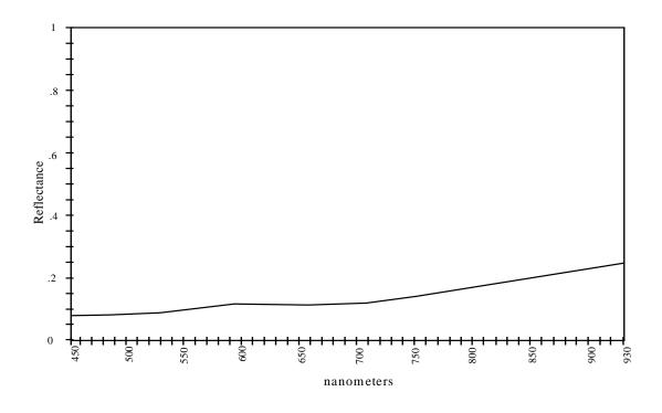
FIGURE C-10. Spectral reflectivity of tree bark.
