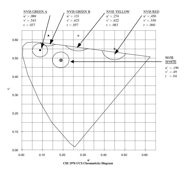
FIGURE 2. NVIS lighting color limits.
