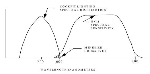
FIGURE C-2. Conceptual diagram of the spectral distribution of NVIS-compatible lighting.
