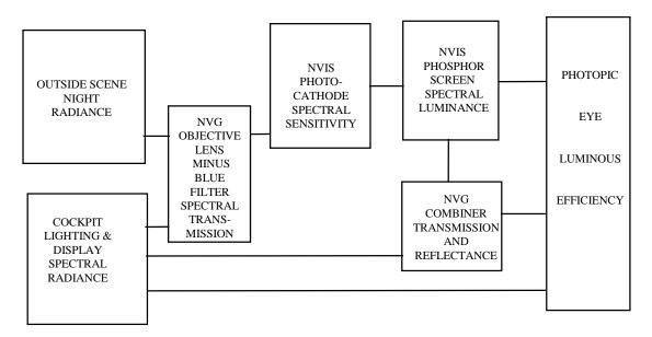
FIGURE C-3. NVIS interfaces.
