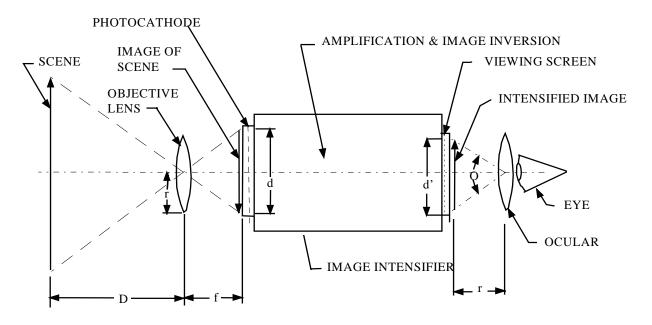
FIGURE C-1. Diagram of an image intensifier.
