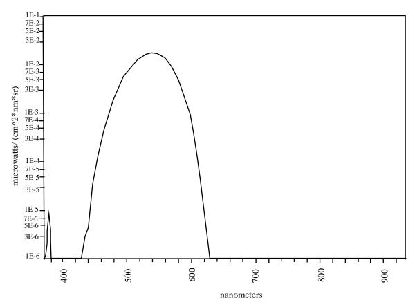
FIGURE B-1. Spectral output of example signal at rated drive conditions (6.1108 cd/m²) (1.7839fL).
