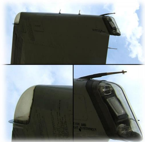
Figure 1: EAA AirVenture Show 2012 - plastic lens left side, glass lens on right side of image
